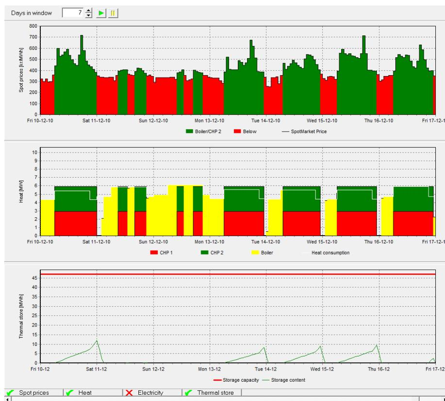
**Figure 4:** This figure shows a simulation in energyPRO of a spot market operation of a typical Danish CHP-plant with a big thermal store in a week in December. In hours with low spot prices the boiler will produce the heat.
