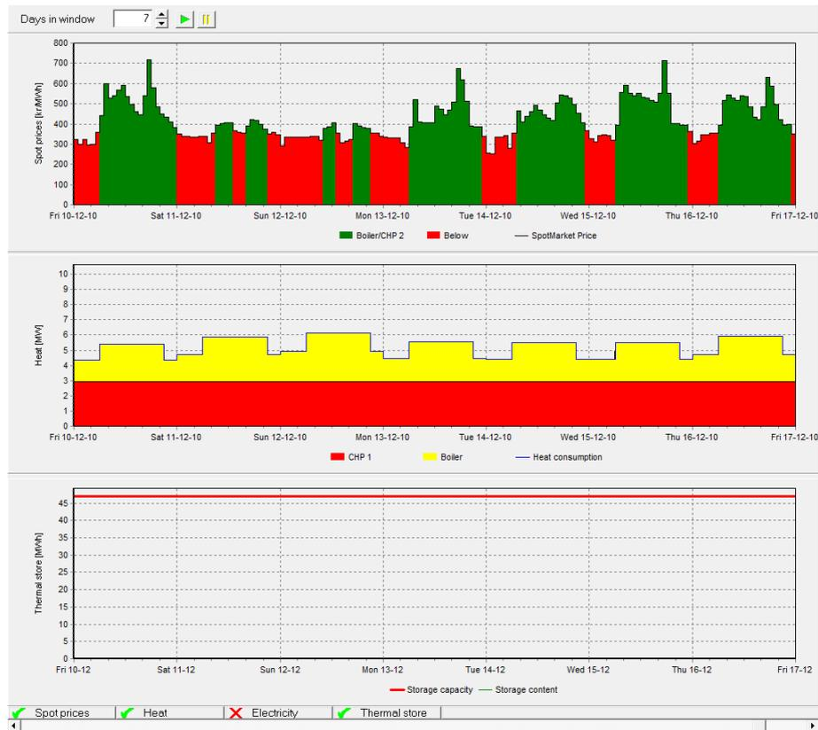
**Figure 5: In this figure is shown the simulated operation of the CHP-plant with a big thermal store in the same week in December. But the operation is planned so that only one of the CHPs is operated in the spot market.**
