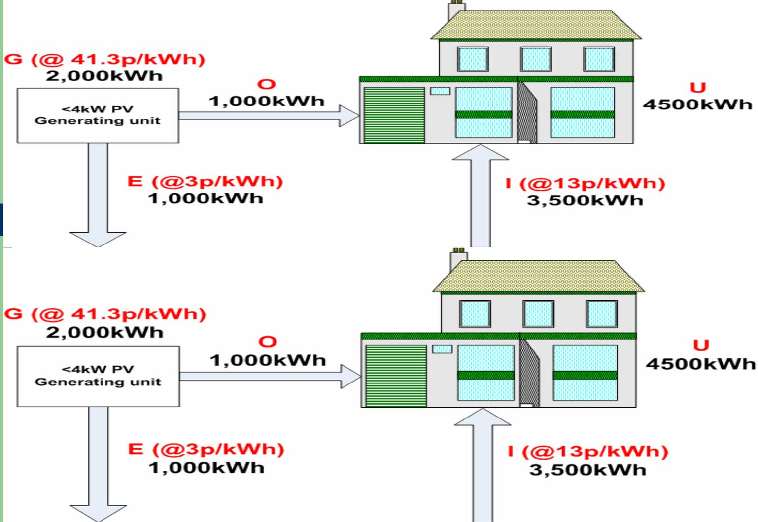
In this illustrative example, the site generates (G) 2,000 kilowatt hours (kWh) per annum (here a retrofitted <4kW solar PV panel) which is metered using the site's generation meter
